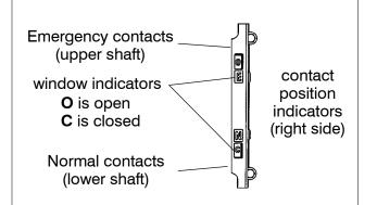
Figure 1-3. Contact position indicators on 150–600 amp. J–design transfer switches . Shown with Emergency open and Normal closed.
